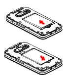
Unclip the cover, then remove the battery.
